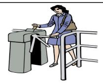
Turnstile: a mechanical gate consisting of revolving horizontal arms fixed to A vertical post, allowing only one person at a time to pass through
